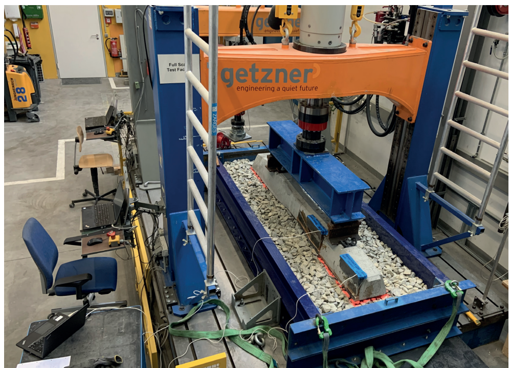
Fig 9. Setup for the entire sleeper test in the ballast box, showing the wired sensor sleeper technology at the nearer end of the concrete sleeper.
