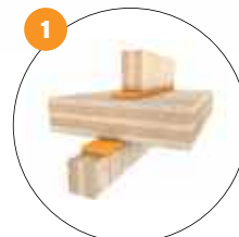
Decoupling of flanking transmission
