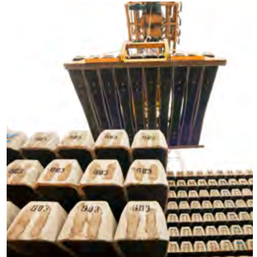
Installation of sleepers at the RailOne plant
